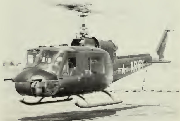
TOW SIGHT —Army UH-1B helicopter takes off on accuracy test of experimental sight for launching TOW missile.
